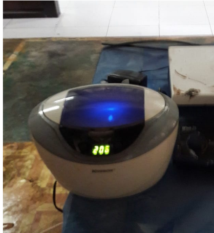
Figure 2. Homogenization process of the PCM–TiO 2 mixture using an ultrasonic bath.
