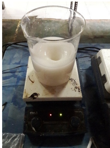
Figure 1. Mixing process of PCM and TiO 2 nanoparticles using a magnetic stirrer.
