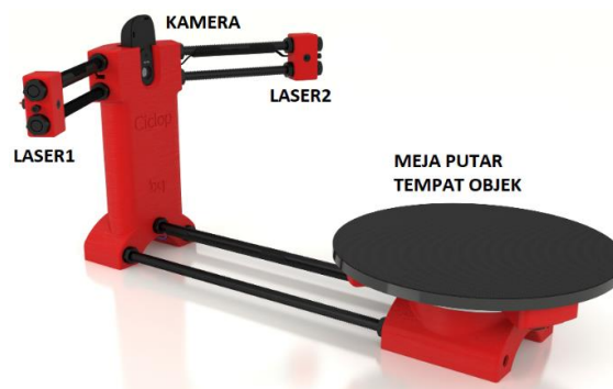
Gambar 1. 3D Scanner Laser Triangulation BQ Ciclop
